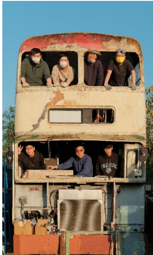
Photos 5 to 6: HSUHK faculty and students scrape away old paint and resand the bodywork of the vintage Leyland Victory Mark II bus during the restoration works.
