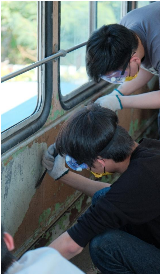
Photos 5 to 6: HSUHK faculty and students scrape away old paint and resand the bodywork of the vintage Leyland Victory Mark II bus during the restoration works.
