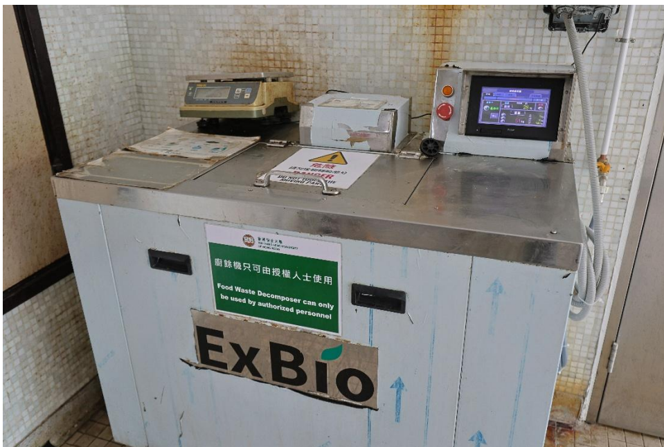
Photo 4: HSUHK installs a food waste decomposer in M canteen to minimise landfill waste.
